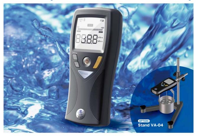
The VT-05/06 is designed for quality control applications in the manufacturing process of industrial products such as petrochemicals, paint, and adhesives, as well as foodstuffs. Viscosity measurements covering a wide range are possible, such as gear oil used in construction machinery. Measurement is performed by simply submerging a rotor in the fluid. The resistance to rotor movement caused by the viscosity (torque) is measured to obtain direct readings.
