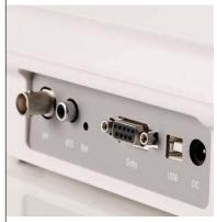
The FiveEasy Plus series meters allows data to be exported either directly to a printer or a PC for further processing using its RS232 or USB ports.
